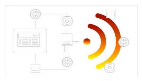
All devices have a notational range of 200m in free air, but the system is supported by an Expander Module to enhance transmission strength in
